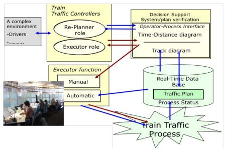
Figure 3. A schedule of how the interaction between different parts of train traffic controlling.
